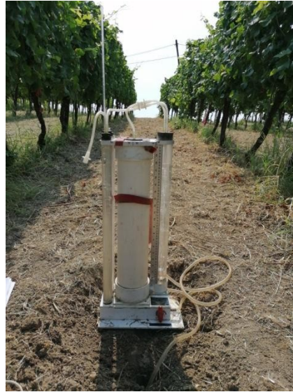
Fig. 24 Field measures of hydraulic conductivity using a constant head permeameter (SMV demo farm).
